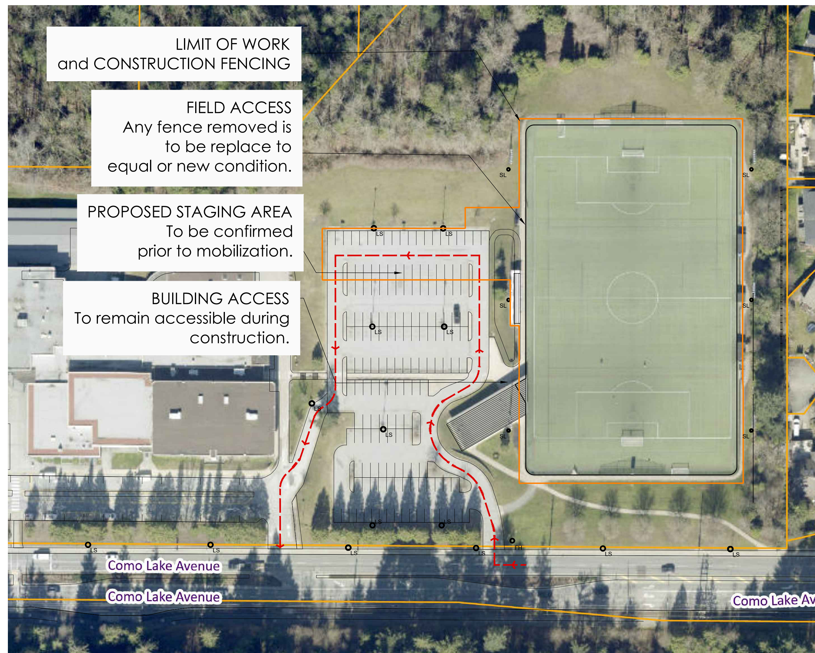
1 ACCESS / STAGING AREA LOCATIONS SCALE - N/A
