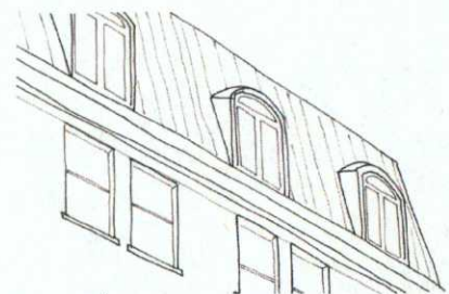
Demonstrates a contemporary mansard roof with dormers
