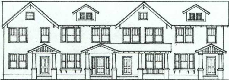
Demonstrates a consistent rhythm across the façade and vertical orientation of the windows
