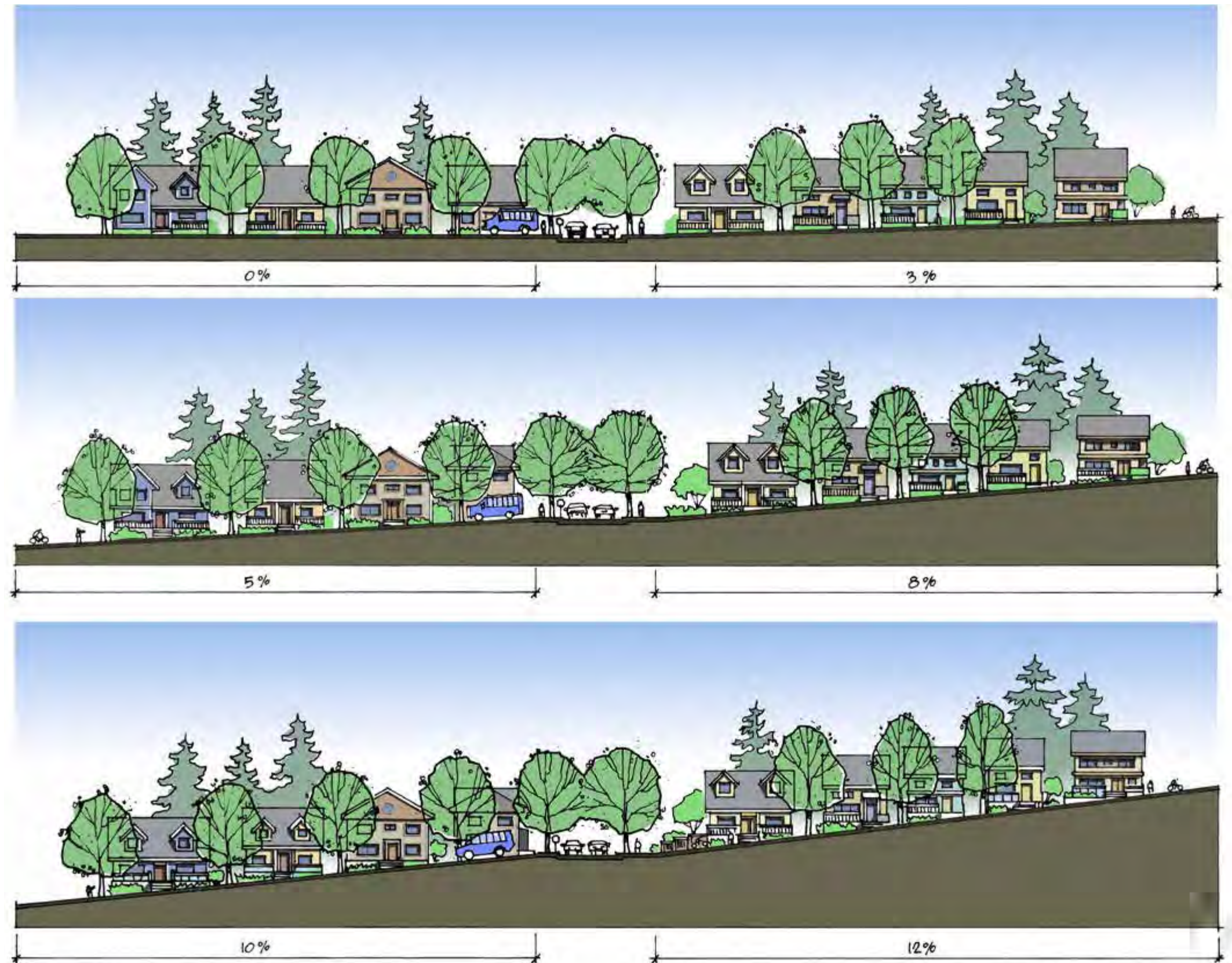
FIGURE 20: ROADWAY GRADES IN THE NBV AREA
